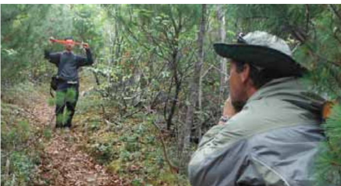
USFS Trails Expert works with a volunteer from the Great Baikal Trail to measure the incline on a section of trail in the Barguzinski Nature Preserve.
